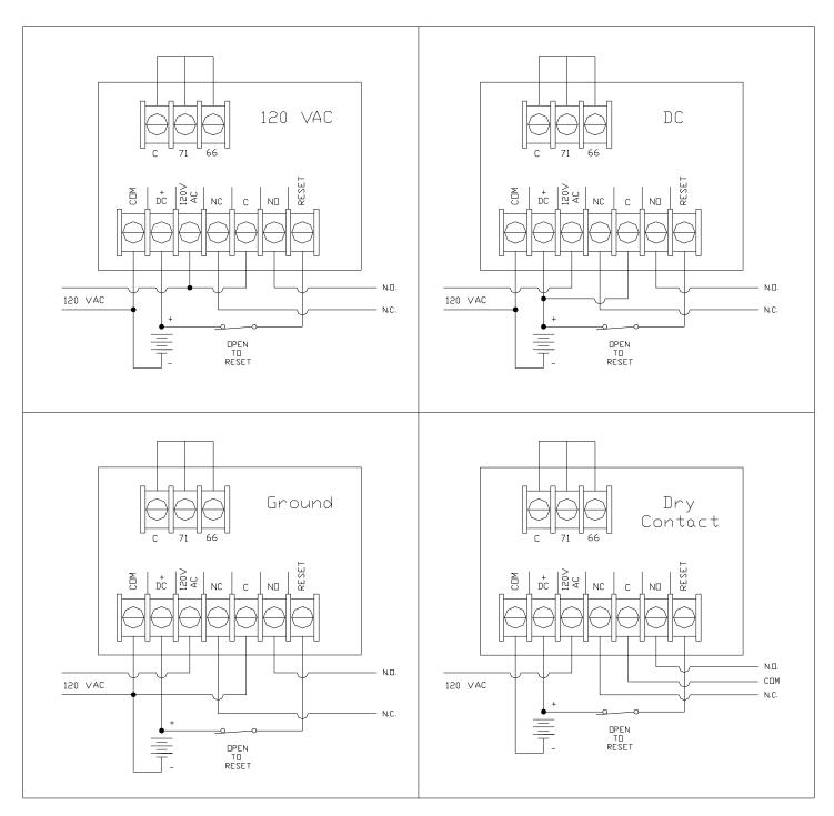
Note: Install jumper between common © and 66 or 71 to select trip frequency.
